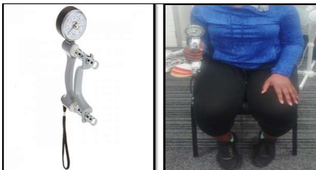
Figure 3.8 Saehan hydraulic hand dynamometer
