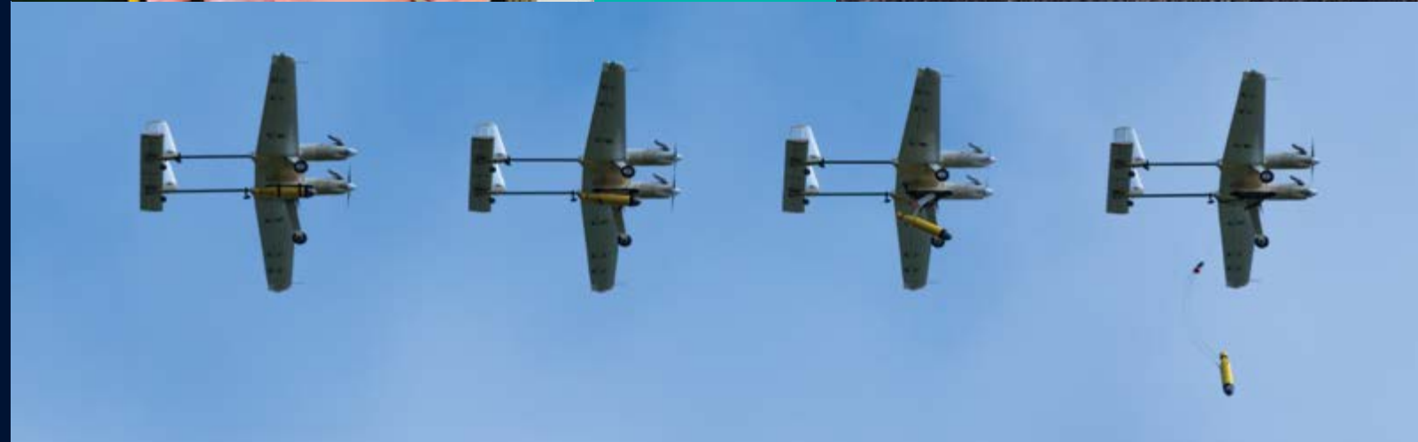
ecoSUB air launch from unmanned aircraft. Photo: ecoSUB
